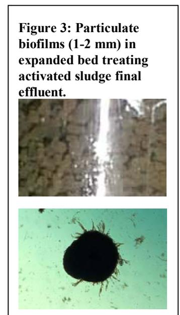
Our technology is a method of process intensification that is based on the natural immobilization of microbes that grow as biofilms on small particles of glassy coke (Fig. 2) and are retained in the bioreactor. These bioparticles (Fig. 3) provide 1,800 m<sup>2</sup> of superficial surface area per m<sup>3</sup> of expanded bed and it is this massive surface area of active biofilm that lies at the heart of our highly effective bioprocess technology.
